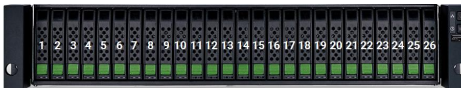
Figure 2-4 System Disk Drive Numbering for the XCubeDAS Series
