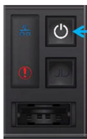
Figure 3-17 Press the Power Button One Time to Power on the System
