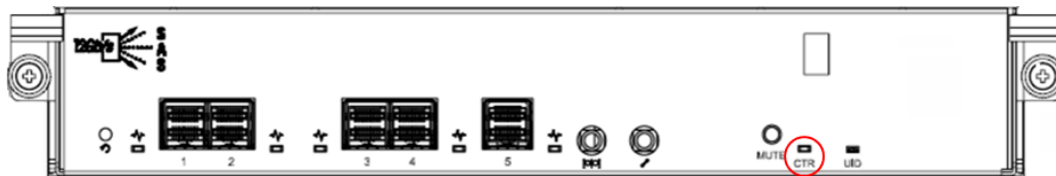
Figure 6-1 Warning Message of Controller Module by the Status LED
